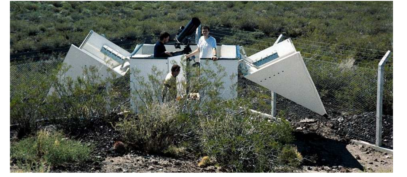
FRAM is part of the Pierre Auger cosmic-ray observatory (Pierre Auger Collaboration 2005), and its main purpose is to immediately monitor the atmospheric transmission. FRAM works as an independent, RTS2-driven (Kubánek et al. 2004), fully robotic system, and it performs a photometric calibration of the sky on various UV-to-optical wavelengths using a 0.2 m telescope and a photoelectric photomultiplier. As a primary objective, FRAM observes a set of chosen standard stars and a terrestrial light source to obtain extinction coefficients. Additionally, FRAM is able to follow GCN alerts, using its wide-field camera with a fixed R -band filter.
