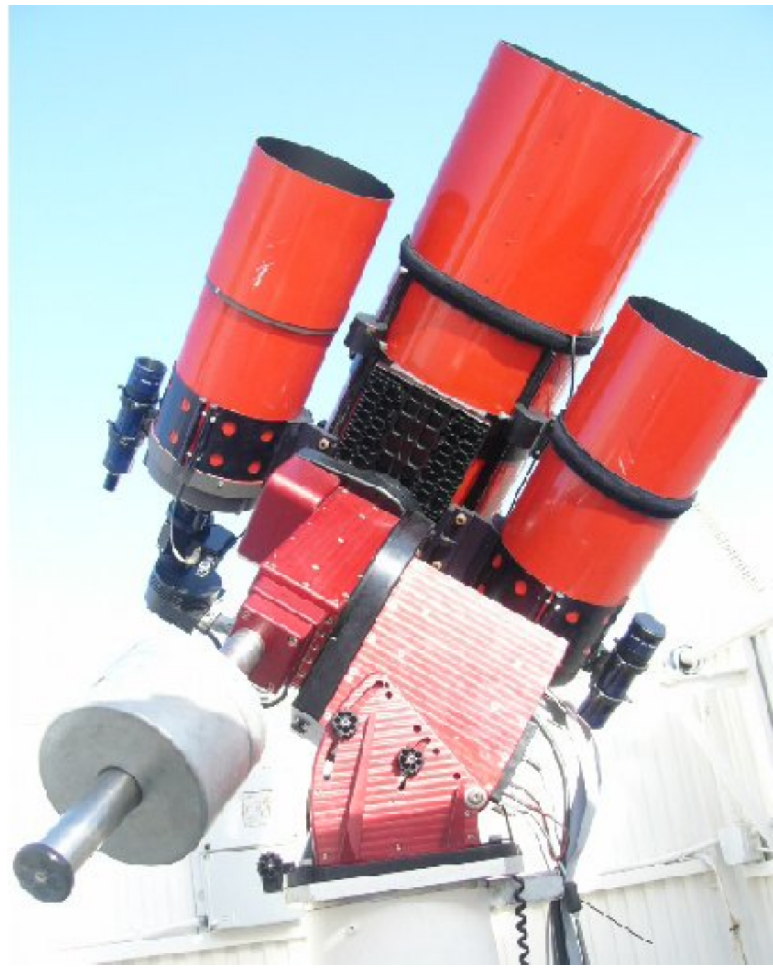
Figure 1: BOOTES-1B: the triple mount with one 30 cm and two 20 cm telescopes.
