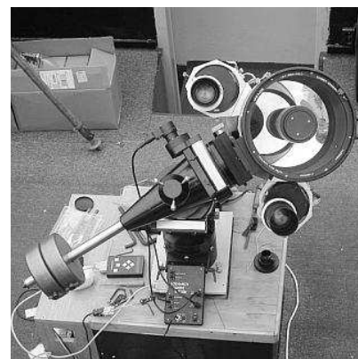
Fig. 1. BART with the wide-field cameras atop the 25 cm telescope.
